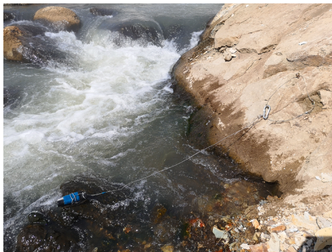
Photo 7. HOBO U20+U24 setup for long-term (month) before bottom installation at section #1 (photo April 21, 2019, Kiryukhin A.V.). Pair of HOBO U20 used for pressure/water level measurements, HOBO U24 was used for specific electro-conductance and temperature measurements.
