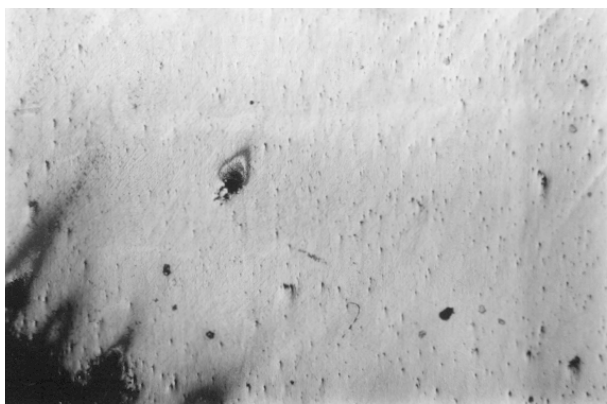
Fig. 3. Surface morphology of 50Ti44Ni5Cu1Mo alloy after polarization test (x 50)
