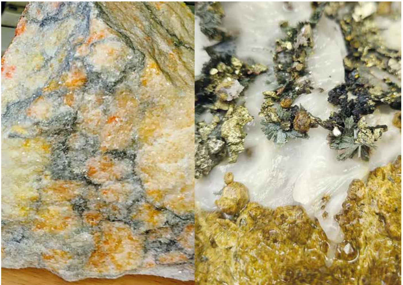
Fig. 2 Marble breccia with realgar and orpiment, the Vorontsovskoe gold deposit (left); skarn with druse cavities filled with the crystals of grossular, pyrite, chalcopyrite, radial fibrous hedenbergite and calcite, the Severopeschanskoe deposit (right). Photo by E. Shagalov
