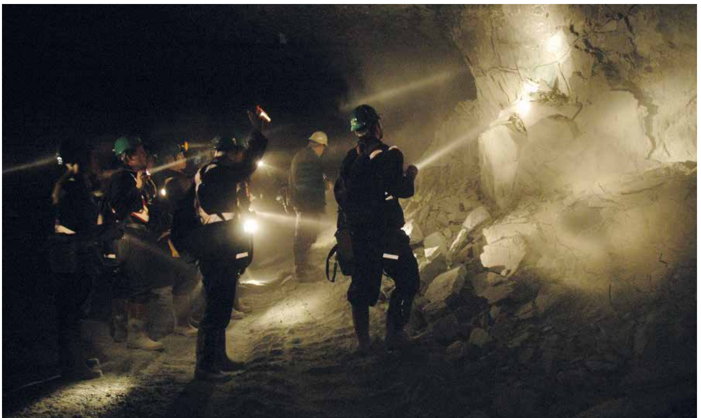
Fig. 3 Participants of the field trip to Cu-Ag Rudna mine during the first chapter meeting in 2009. On the right, typical ore hosting series consisting of Weissliegend sandstone, thin Kupferschiefer layer near roof and Zechstein carbonates above
