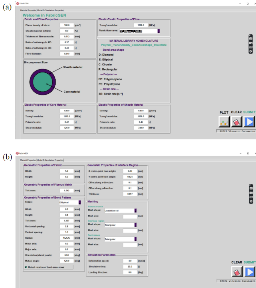
Fig. 4.3 Sections of FabricGEN : (a) materials properties; (b) model and simulation properties [8]
