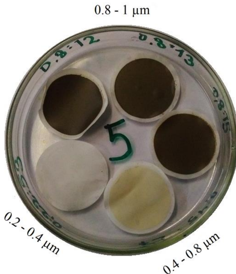
Figure 1 – Problem: clogged filter pores with a pore diameter of 1 \mu\text{m} .
