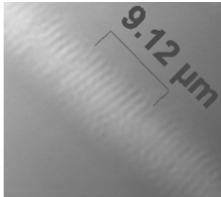
Fig.3. Self-organizing grating inscribed by un-modulated femtosecond beam with wavelength of 400 nm and repetition rate of 1 kHz.
