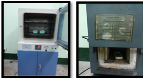
Fig.5. Drying and Calcination Magnesium Hydroxide Precipitate
