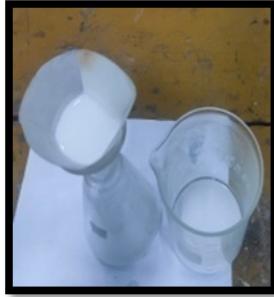
Fig.4. Washing and Filtration of Magnesium Hydroxide Precipitate
