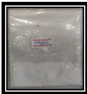
Fig.6. Final Product Magnesium Oxide Nanoparticles Powder
