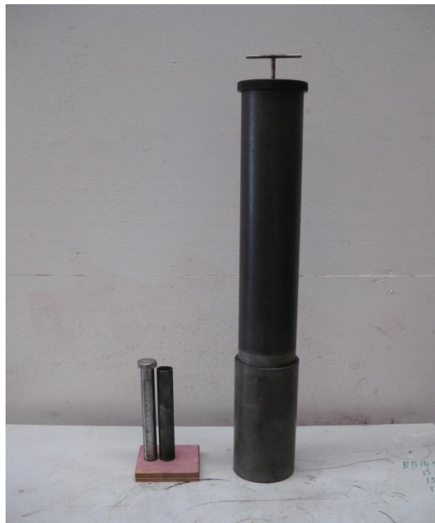
Figure 9: Drop hammer equipment – measuring cylinder with scale and tube with drop hammer
