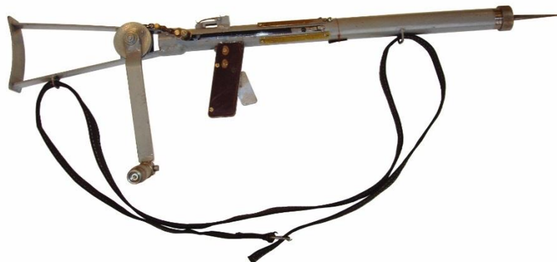
Figure 8: Russian penetrometer gun for q index test
