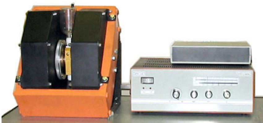
Figure 2. Compact EPR equipment
