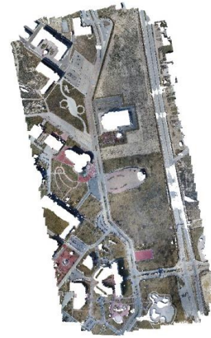
Fig. 3 Point cloud filtered by CSF. (Ground point)
