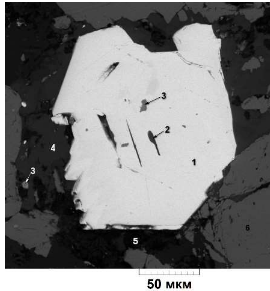
Fig. 3. Hydroxyplumboroméite (1) associated with epidote (2), mineral of the rutil-tripuhyite series (3), calcite (4), quartz (5) and tilasite (6). Sample 9999B. BSE image.
