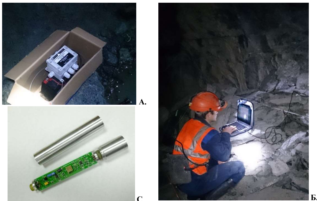
Fig. 1. Appearance of WSN equipment. A- in the box the transmitting unit and the battery; B - The author of the article downloads the current data from the hub to the laptop; C- Hydrogen sensor with the protective case removed. A sensor chip and a connector for cable are visible.
