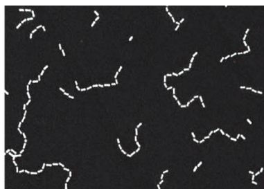
Figure 1. Transmission electron microscopy image of linear nano-polymer chains self-assembled from gold nanorods end-terminated with polystyrene molecules
