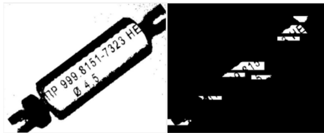
Fig.1: The illustration of the drawback of text area selection by mathematical morphology methods, when the label is rotated by an angle of more than 20^\circ
