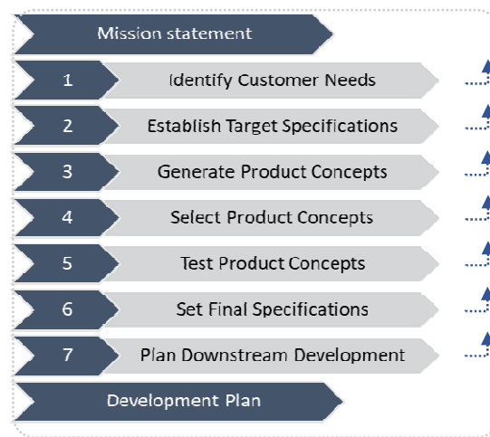
Fig. 1: Product specifications within the concept development process [adapted from Ulrich K.T. and Eppinger S.D. (2012)]
