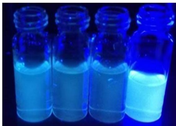
Figure 1: Carbon quantum dots under UV-lamp.
