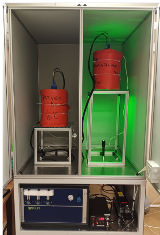
Figure 1: Experimental setup for the dispersion of LASER beams in a batch reactor with bacteria mixtures.
