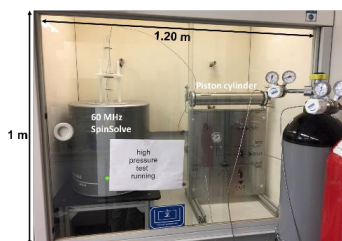
FIGURE 1. Photograph of the presented HP setup inside a chemical laboratory fume hood.
