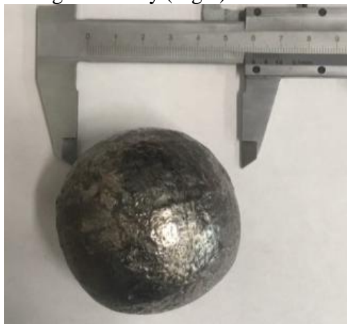
Figure 1 – Cast-iron grinding media
