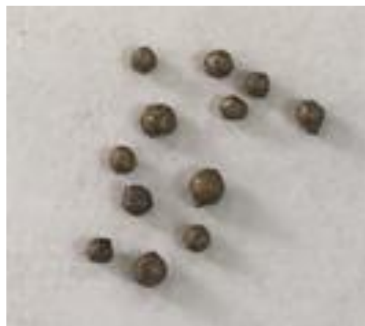
Figure 2 – Proppants with a diameter of 0.6 – 1.0 mm
