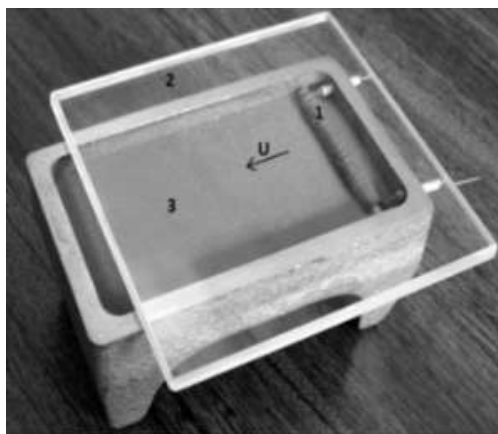
Рис 1. This figure illustrates a particular combustion experiment [2]. Titanium is poured into the boat and covered with quartz glass plate. Titanium is ignited in air, which passes through a narrow slit. An unusual type of "vibrating" combustion is observed.
