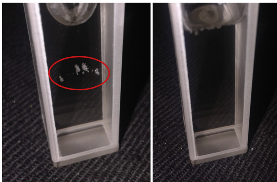
Fig. 6. Hydro-gel (22% wt. Pluronic) with SWCNTs after optical breakdown (encircled) by high-power laser irradiation (left), and the same sample regenerated by temperature drop down to 5°C (duration 10 min) and subsequent gelation (right); in both cases pictures are taken at room temperature.
