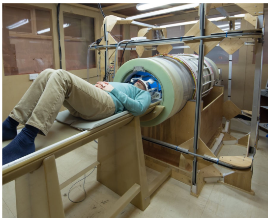
Figure 1. 0.2 T FFC-MRI scanner at the University of Aberdeen
