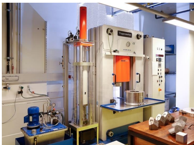
Figure 1: 1000 t multianvil high-pressure device for the realization of extreme pressures and temperatures.
