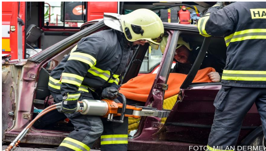
Fig. 2 Pruning post B by hydraulic equipment [5]
