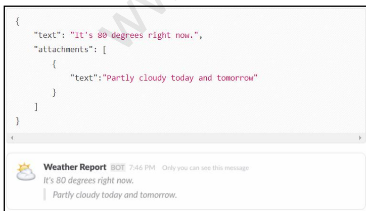
Figure 4. Sample Slash Command JSON Response and how it looks in Slack
