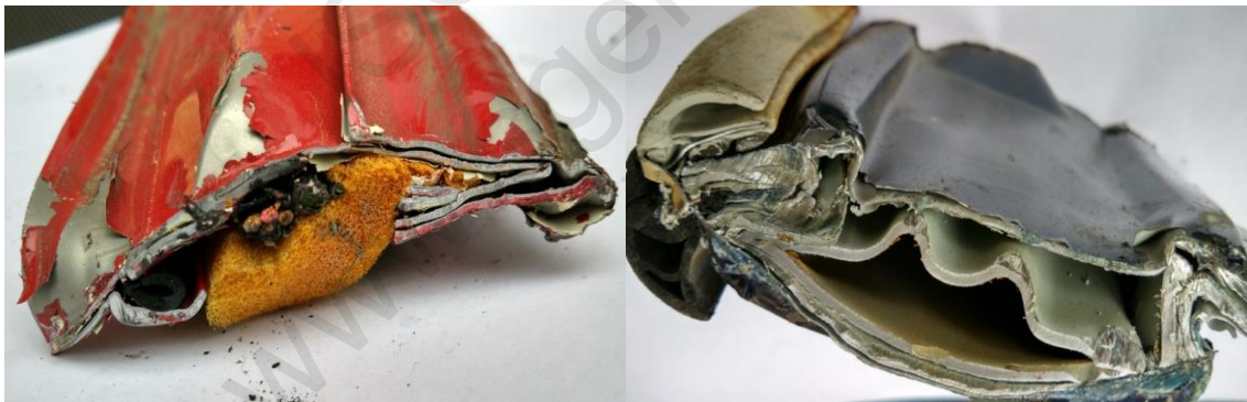
Fig. 3 Post A (left) and Post B (right) after execution cutting works by hydraulic equipment
