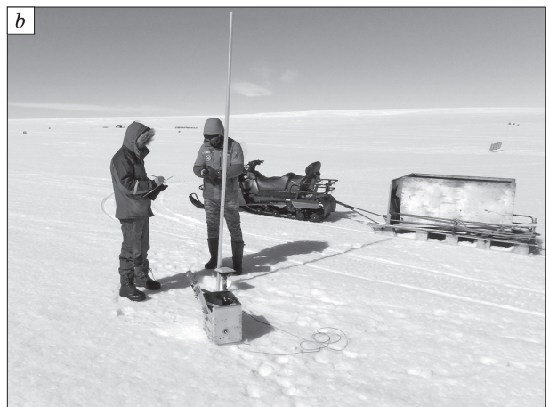
Fig. 3. Photograph of the damaged marker stake (a) and measuring procedure for the position and height of maker stakes (b).
