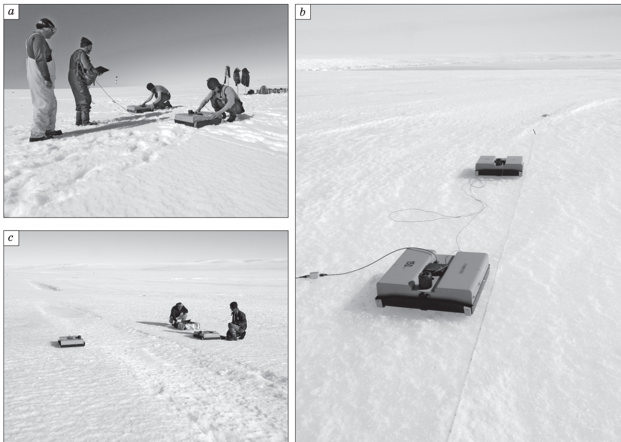
Fig. 6. Performing CDP multi-offset soundings.
