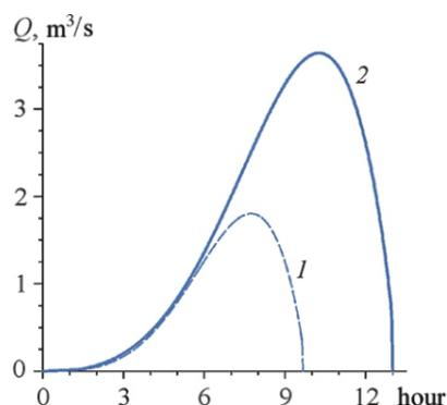
Fig. 3. The calculated hydrographs for the outburst flood on (1) Lake Discussion and (2) Lake Progress.
