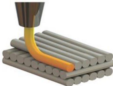
FIGURE 1. FDM Printing Material Structure (From https://3dprint.com/wp-content/uploads/2015/02/mat.png )
