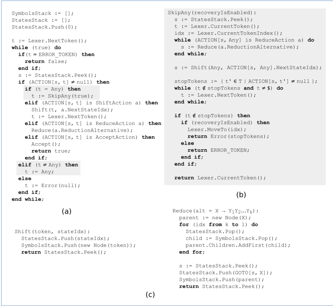
Fig. 2. Modified LR algorithms: (a) Modified LR(1) parsing algorithm, (b) “Any” processing algorithm, (c) Shift and reduce algorithms.
