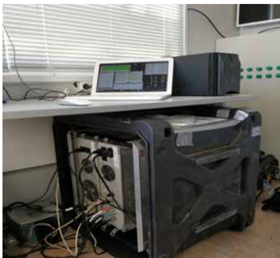
Fig. 1. Sea Sonde electronic unit
