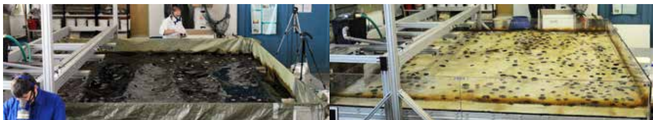
Fig. 1. «Wave pool» after adding bio-sorbents (left) and in 24 hours (right).
