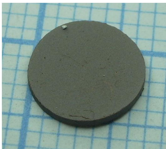
Figure 1. Pellet of highly radioactive Synroc-like titanate ceramic obtained after sorption of real liquid HLW on LHT-9 followed with cold pressing and sintering in air at 1200°C during 2 hours. Scale grid is 1 x 1 mm.
