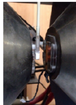
FIGURE 6. Sample in a variational magnetometer.
