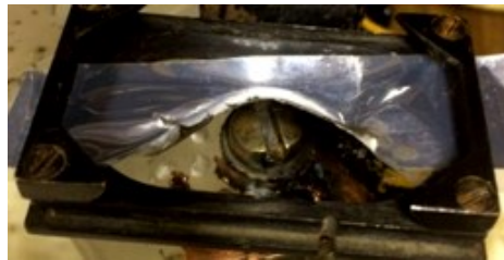
FIGURE 9. Results of interaction of a jet with a thin membrane.
