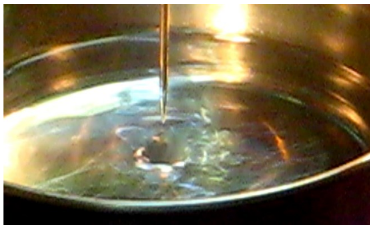
FIGURE 3. Appearance of a cavity over the alcohol surface, metallic cavity, a distance between the upper electrode and a surface is 5 mm. Positive corona.
