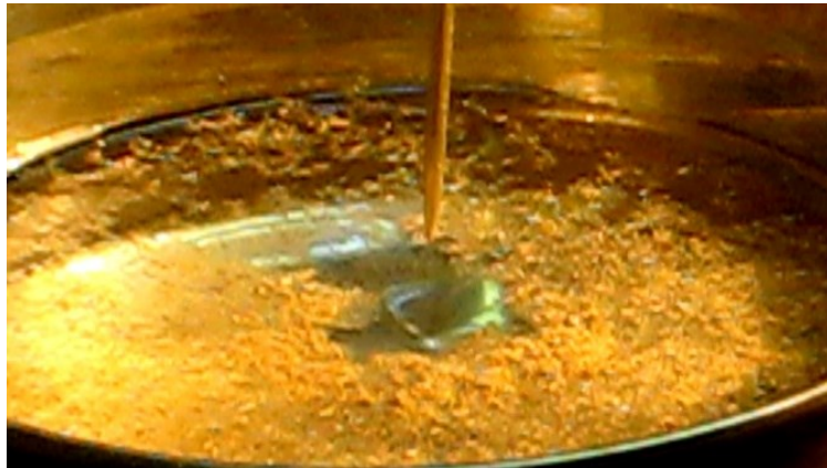
FIGURE 2. Appearance of a funnel over the water surface covered with the wooden powder, metallic cavity, a distance between the upper electrode and a surface is 5 mm, electrode is in central position, positive corona.
