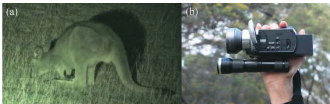
Fig. 8. Night observations and registration of behaviour of wild animals: a — an eastern grey kangaroo in infrared light, b — a video camera in the NightShot mode equipped with an infrared illuminator (Bars IK-K3).
