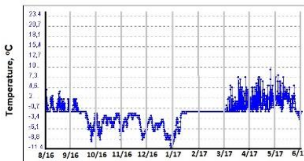
Fig 2: Soil temperatures (0-10 cm) over the season August 2016-June 2017 as collected from permanent monitoring plot at Erkuta river derived from thermologgers
