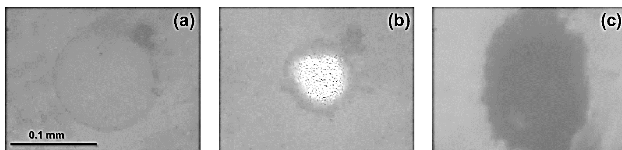
Fig. 1. Microphotographs of the sample (80 wt.% basalt + 20 wt.% C_2H_2O_4 ), taken during experiment in the diamond anvil cell: (a) compressed mixture at 25 °C and 0.8 GPa; (b) decomposition of oxalic acid, 395 °C and 4.0 GPa; (c) coexistence of opaque polymeric phase and silicate phases at 900 °C and 4.7 GPa.
