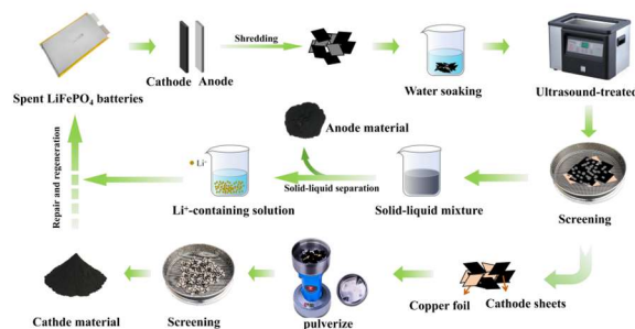
• Figure 1. Flowchart for the efficient separation of anode and cathode materials using the water soaking method.
