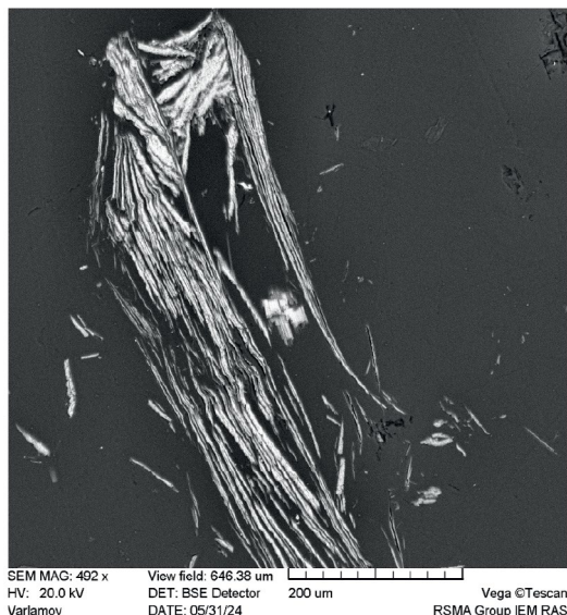
Fig. 3. Fibrous aggregate of NHTS intergrown with unidentified hydrous Na, K, Ca-silicates. SEM (BSE) image of a polished section
