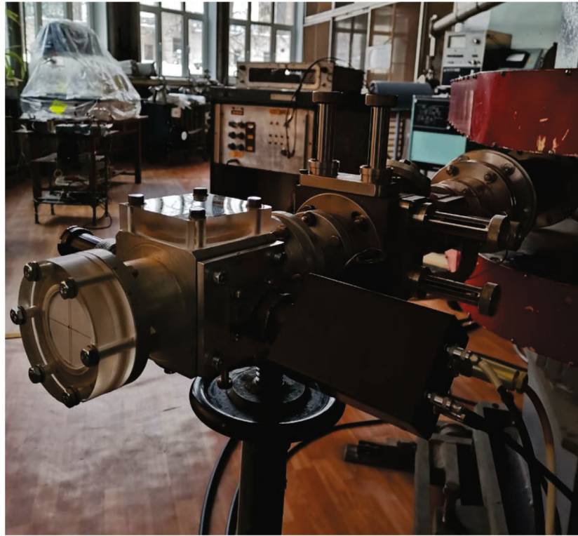
Fig. 4. Multisensor system for monitoring beams of charged particles and heavy ions, mounted on the ion guide of the U-120 Cyclotron of the Ioffe Institute.
