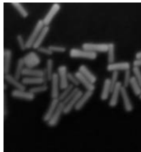
Figure1 (b). Scanning electron microscope image of rod-shaped gold nanoparticles.
