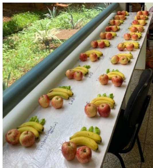
Figure 2. Storage and measurement of fruits/vegetables with/without deposited nanodispersions to measure the process of weight loss.
