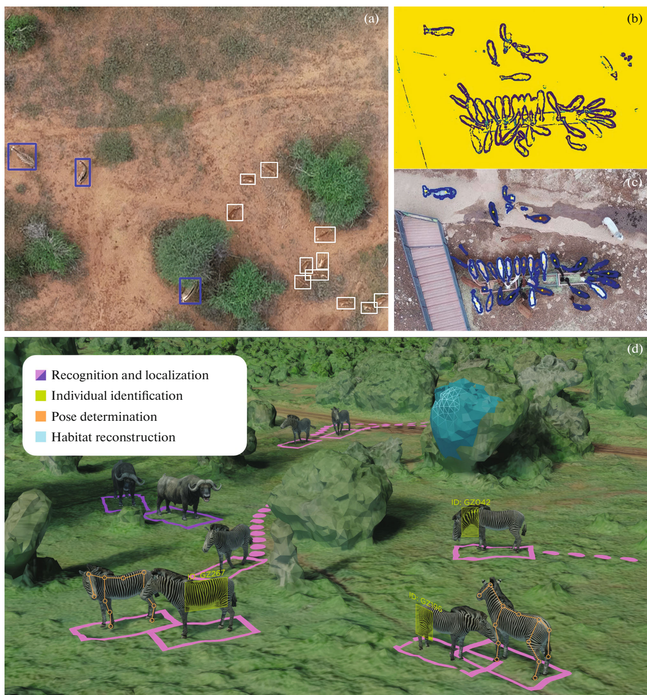
Fig. 3. Using computer vision algorithms to analyze materials obtained from UAVs. (a) Simultaneous automatic detection and tracking of two ungulate species with visualized object bounding boxes (bbox) for two video frames using trained models (zebras, blue; impalas, white). An example of automatic detection of animals on a complex background (b) using the Sobel operator function for edge detection and (c) their rendering onto the original image. (d) A summary infographic demonstrating modern capabilities of using computer vision for recognizing the species of mammals and their position in space (purple), tracking their movements (pink), individual identification of individuals (green), categorization of body postures (orange), and reconstruction of habitats, including damaged ones (blue). The illustrations are under an open license for reuse: (a) Koger et al., 2023; (b, c) Lee et al., 2021; (d) Tuia et al., 2022.
