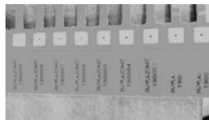
Fig. 13 Seal visualization marked by thermal print and damaged by technical petrol
