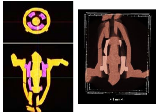
Fig. 8 A cut through seal of the PL type deformed by heat (120 °C) and a 3D model of the destroyed seal
