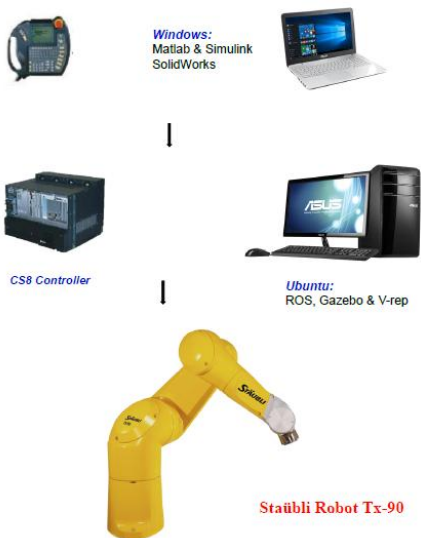
Figure 4: Control Diagram of Stäubli Robot Tx-90
