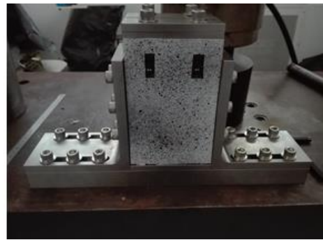
Figure 4. Edge-constraint structure adopted in the experiment
