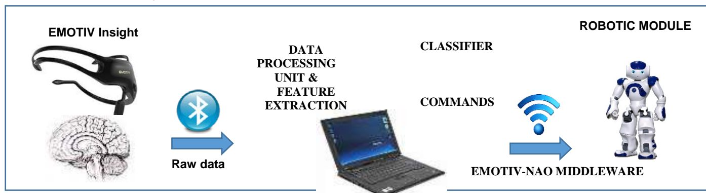
Fig. 3. EMOTIV-NAO wireless framework for developing an EEG based brain-robot interface
