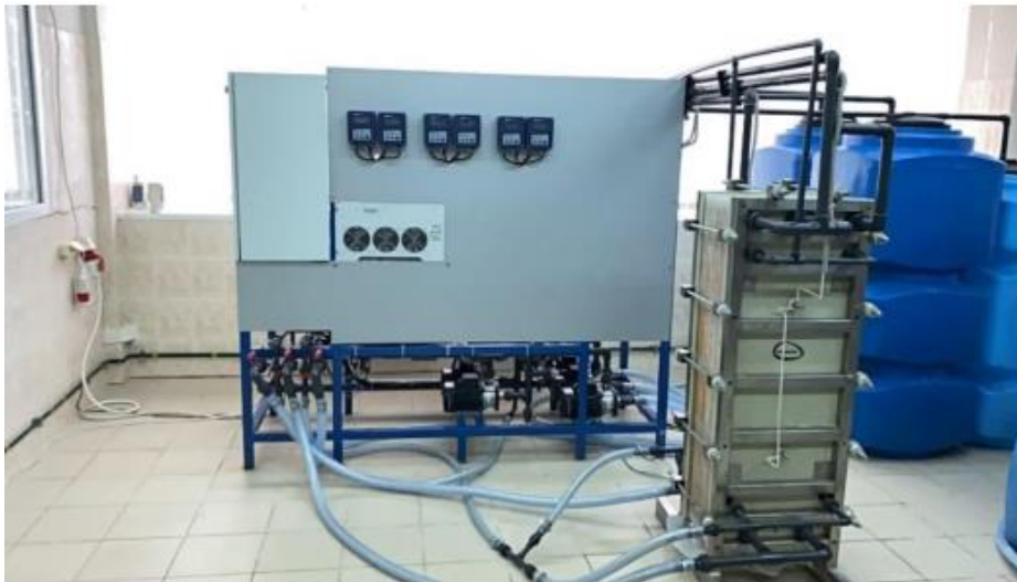
Figure 2 – External view of the developed electromembrane complex in the business incubator of KubSU.
