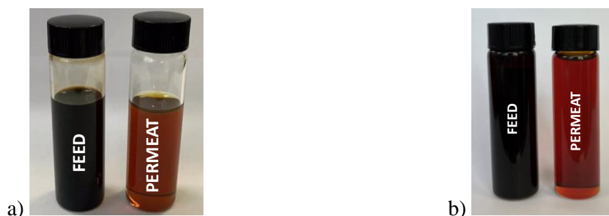
Figure 1. Photographs of the initial mixture and permeate after filtration: (a) oil solutions in toluene with an oil content 100 g/l through a membrane with a pore size of 4 nm; (b) oil through a membrane with a pore size of 21 nm (b).
