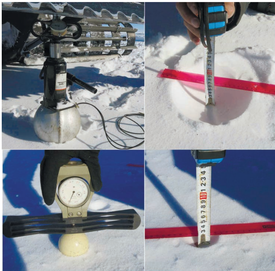
Fig. 8. Scheme of the experiment measuring the strength characteristics of natural snow cover by the Brinell method. The photos are by S.P. Polyakov
