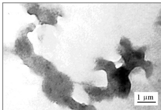
Fig. 3. Solid phase in fuel D (TEM image).
