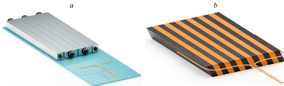
Fig. 1. Structure of a heat flux sensor based on anisotropic thermoelements (a) and on heterogeneous structure of a copper-nickel (b).
