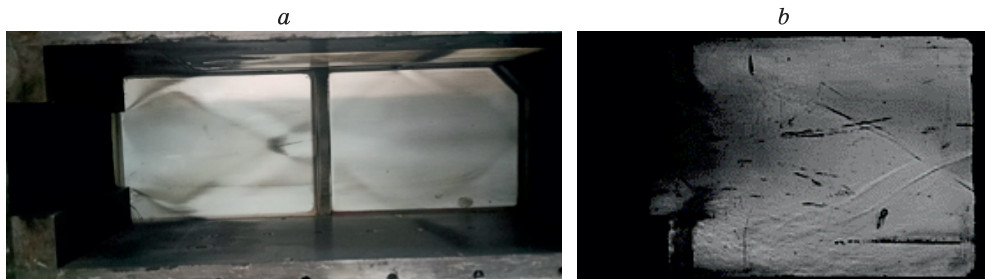
Fig. 1. Photo of the window after run with methane (a) and Schlieren visualization of the initial section of the channel with an air jets behind the back step (b).
