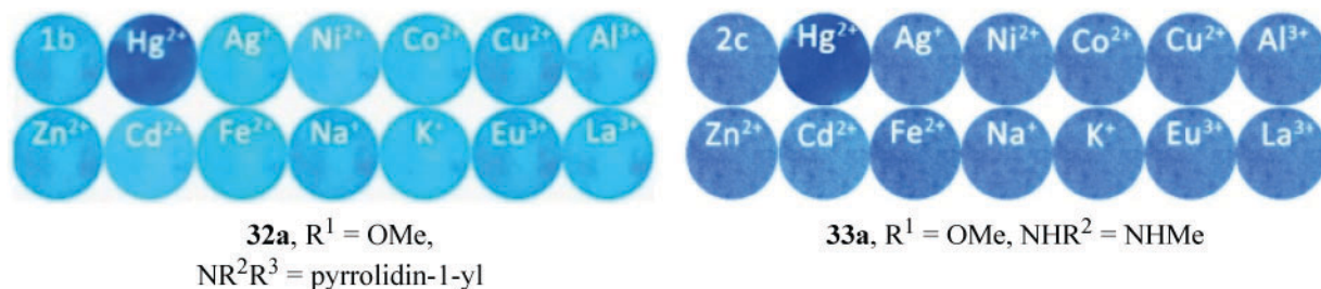
Fig. 13.1. Photographs of the test strips impregnated with a solution of 1,2,3-triazoles 32a and 33a , treated with aqueous solutions of metal ions, under irradiation with a 365-nm UV lamp.
