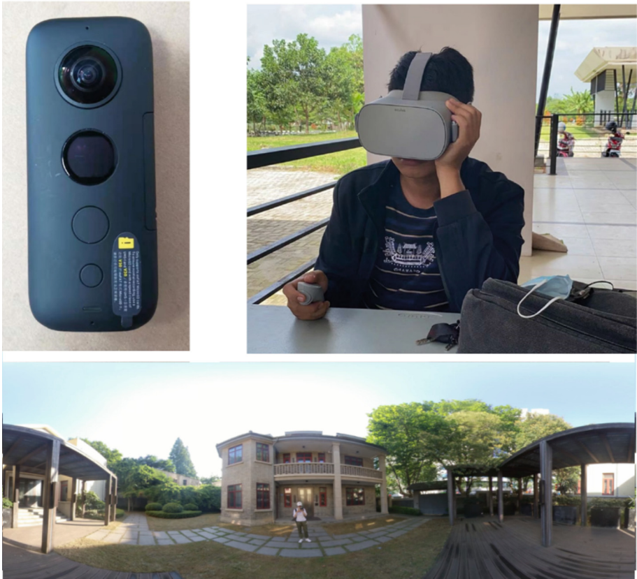
Fig. 2. 360-degree camera to create VR tours, head-mounted display to watch VR tours, and a screenshot of VR tour.
