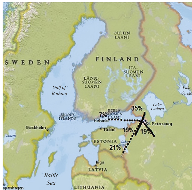
Fig. 5. Clusters of reverse trajectories of air mass movement according to calculation data of the HYSPLIT model for days with high values \sigma_{sp}(550) (more than 70) according to nephelometer measurements.
