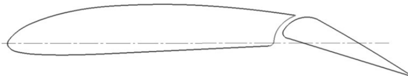
Fig. 1. Model of airfoil CLARK Y+ with deflected flap on \delta_{flap} = 20^\circ .
