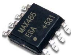
Fig. 2. MAX485 Integrated Circuit with SOP.
