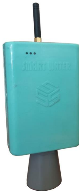
Fig. 10. Industrial example of the smart device for determining water flow.
