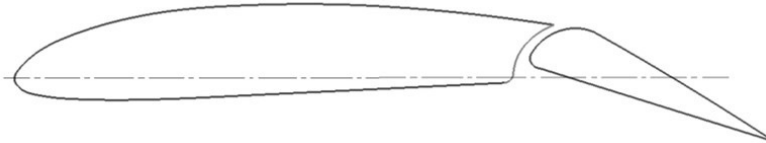
Fig. 1. Model of airfoil CLARK Y+ with deflected flap on \delta_{flap} = 20^\circ .
