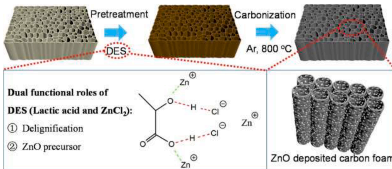
Fig. 6. Schematic illustration of the preparation process of ZnO deposited carbon foam copied from [55]. The figure is taken entirely from the original source.
