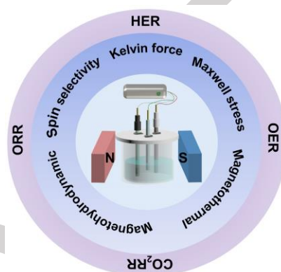
Scheme 1. Possible mechanisms (magnetothermal effect, magnetohydrodynamic effect, Maxwell stress effect, Kelvin force effect, and spin selectivity effect) of magnetic field-enhanced electrocatalysis.
