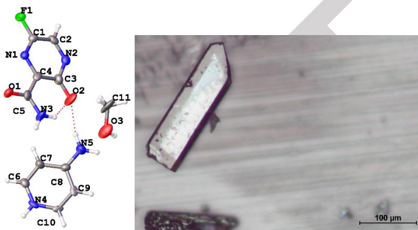
Scheme 1. Fragment of the crystal structure and snapshot of the crystal for the cocrystal of Favipiravir and 4-aminopyridine in methanol.
