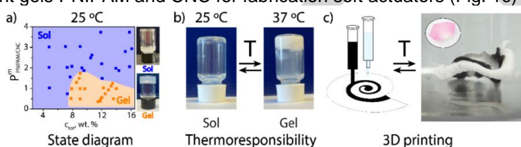
Figure 1. a) state diagram for the mixture PNIPAM/CNC at 25°C; b) appearance of aqueous dispersion of CNC grafted PNIPAM at sol state at 25°C (left) and gel state at 37°C (right); c) rose-petal shape actuation scheme (left) and shape transformation of the material at 37°C (right). Actuation shape transformation inspired by Rosa odorata .
