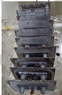
Scheme 1. Samples after exposure to a salt fog chamber
